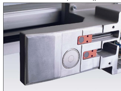
Infrared sensors for edge positioning
